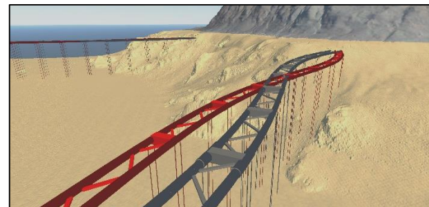
Sulafjorden submerged floating tunnel bridge
