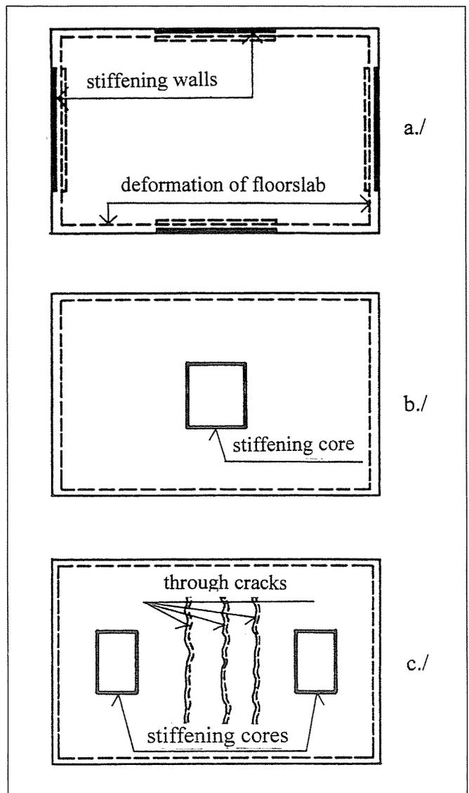
**Fig. 6** Effect of the arrangement of stiffening structures:
