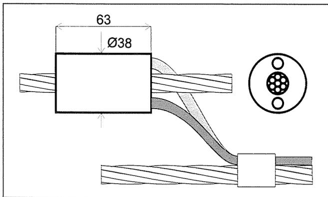
**Fig. 1** Sensors pulled onto tendons built-in UBx type prefabricated, prestressed concrete beams
