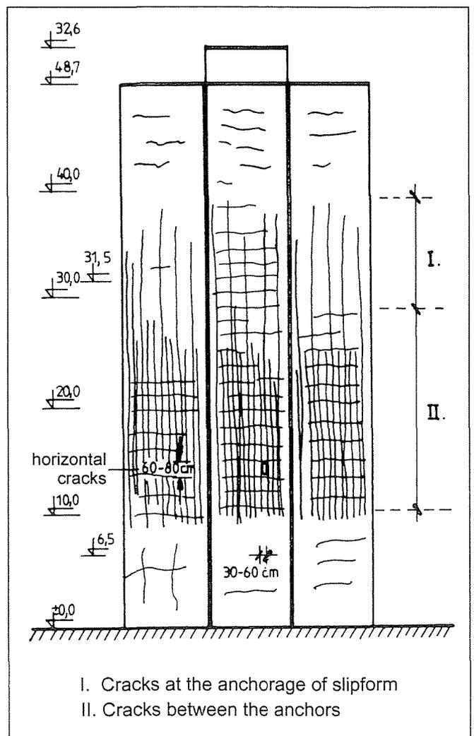
Fig. 3 Characteristic cracks in the silo walls
