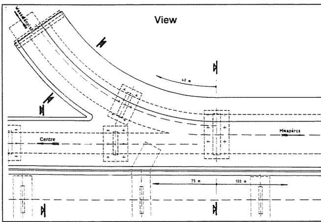
**Fig. 1** Layout of the bridge at the access branch
