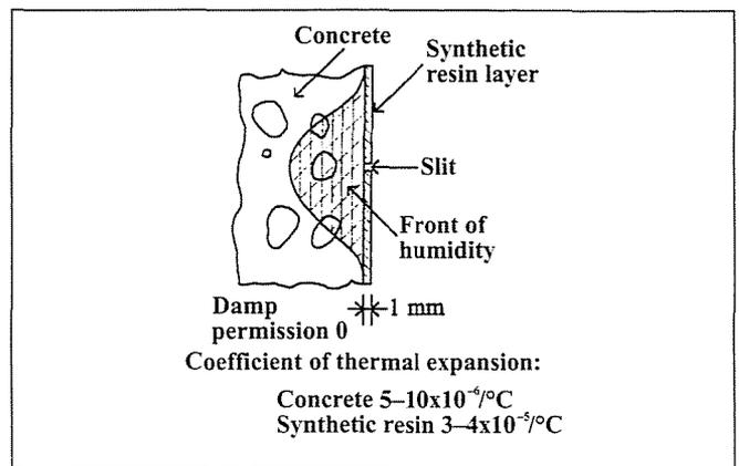
Fig. 4 The water front spreads below the damaged resin layer, it can not dry out
