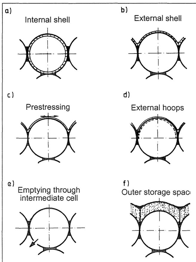
Fig. 4 Methods of strengthening
