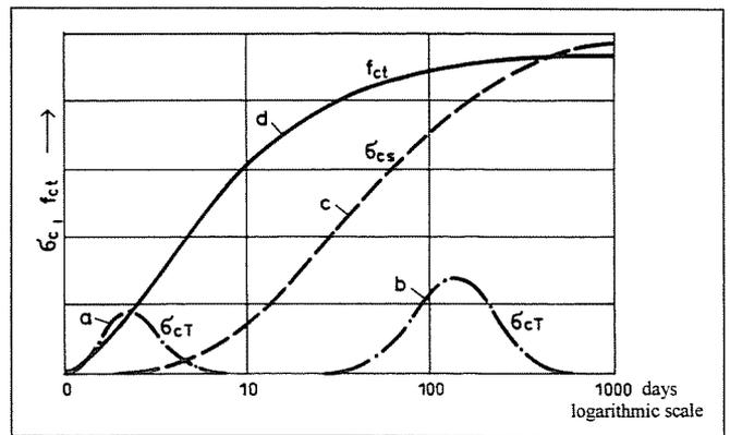
**Fig. 3** Evolution of tensile stresses and tensile strength in the concrete.
