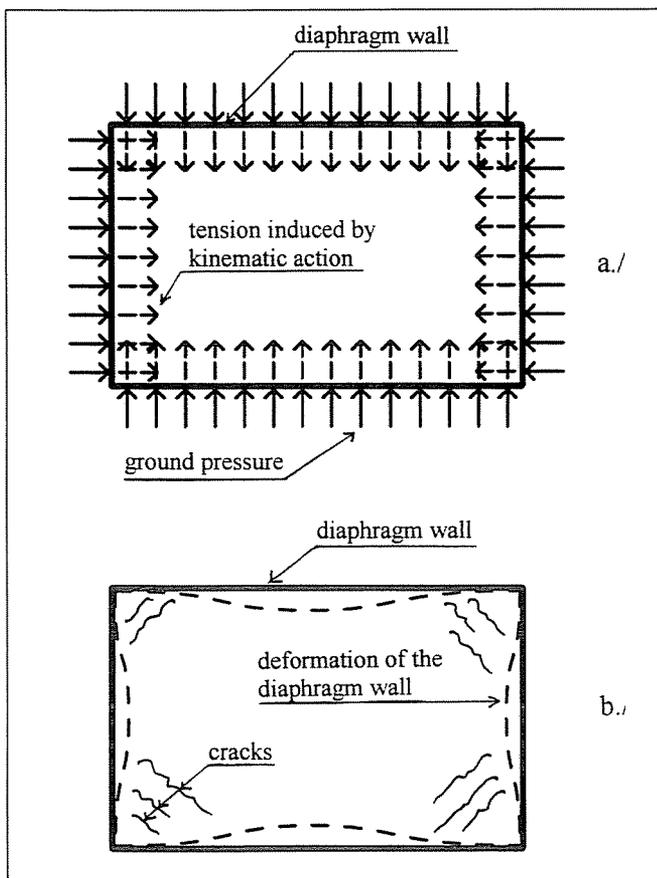
**Fig. 5** Deformation of diaphragm wall
