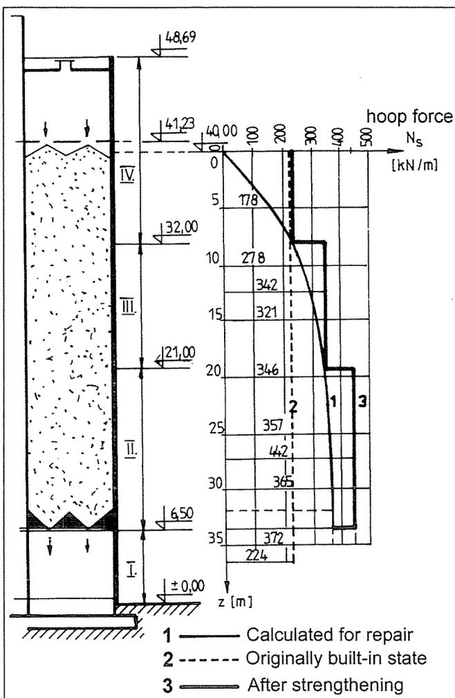
Fig. 5 Limit hoop-forces and ring-forces
