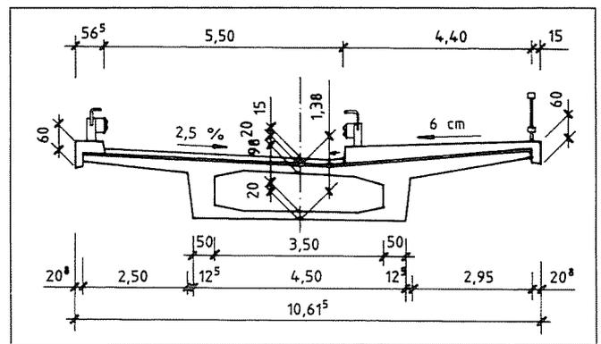
**Fig. 3** Transverse section under the access branch
