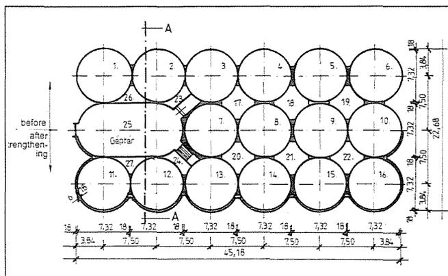
**Fig. 2** Vertical section of the silo
