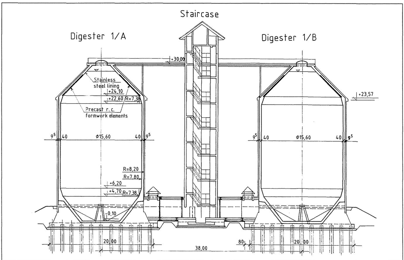
Fig. 2 Perpendicular section of the digesters and stair case
