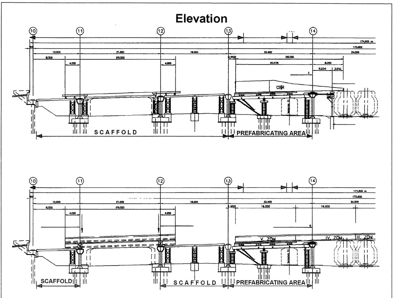
**Fig. 5** Structure built on scaffold and the beginning of incremental launching
