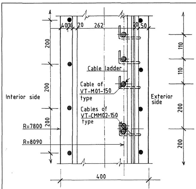
Fig. 4 Reinforcement of cylindrical wall, detail
