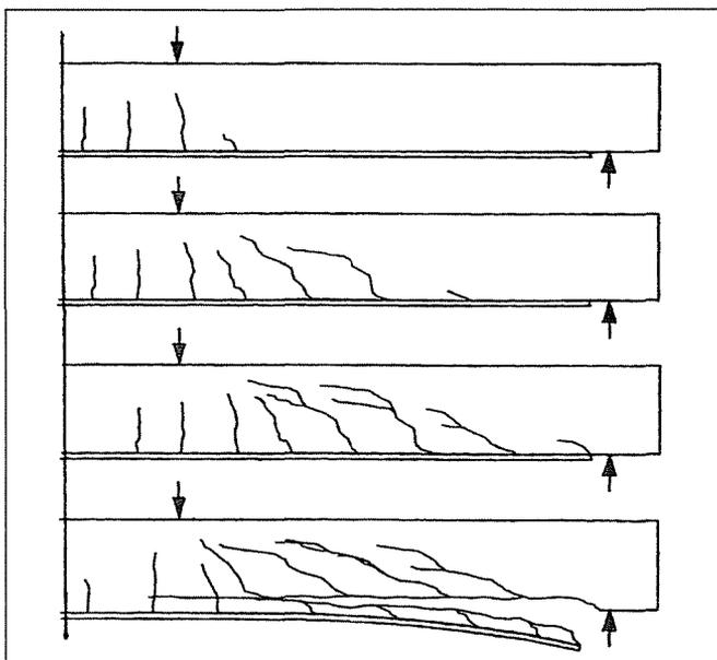
Fig. 11 Anchorage failure (peeling off) (Hollaway and Leeming, 1999)
