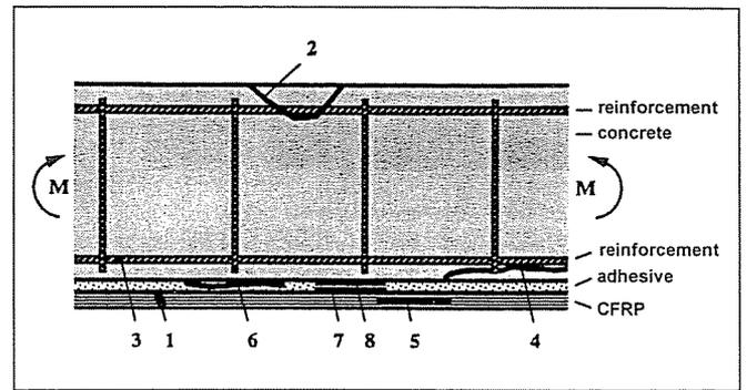
**Fig. 10** Possible failure modes of a reinforced concrete member strengthened by carbon fibres (Deuring, 1993)
