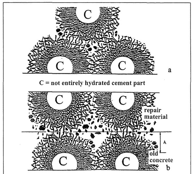
Fig. 2 Sketch of the joint of a silicate frame, a) in a state when they are not completely grown together, b) their principal scheme
