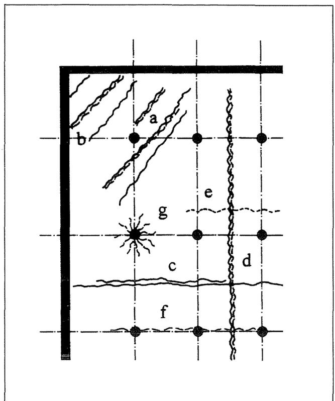
**Fig. 2** Typical floor slabs cracks:
