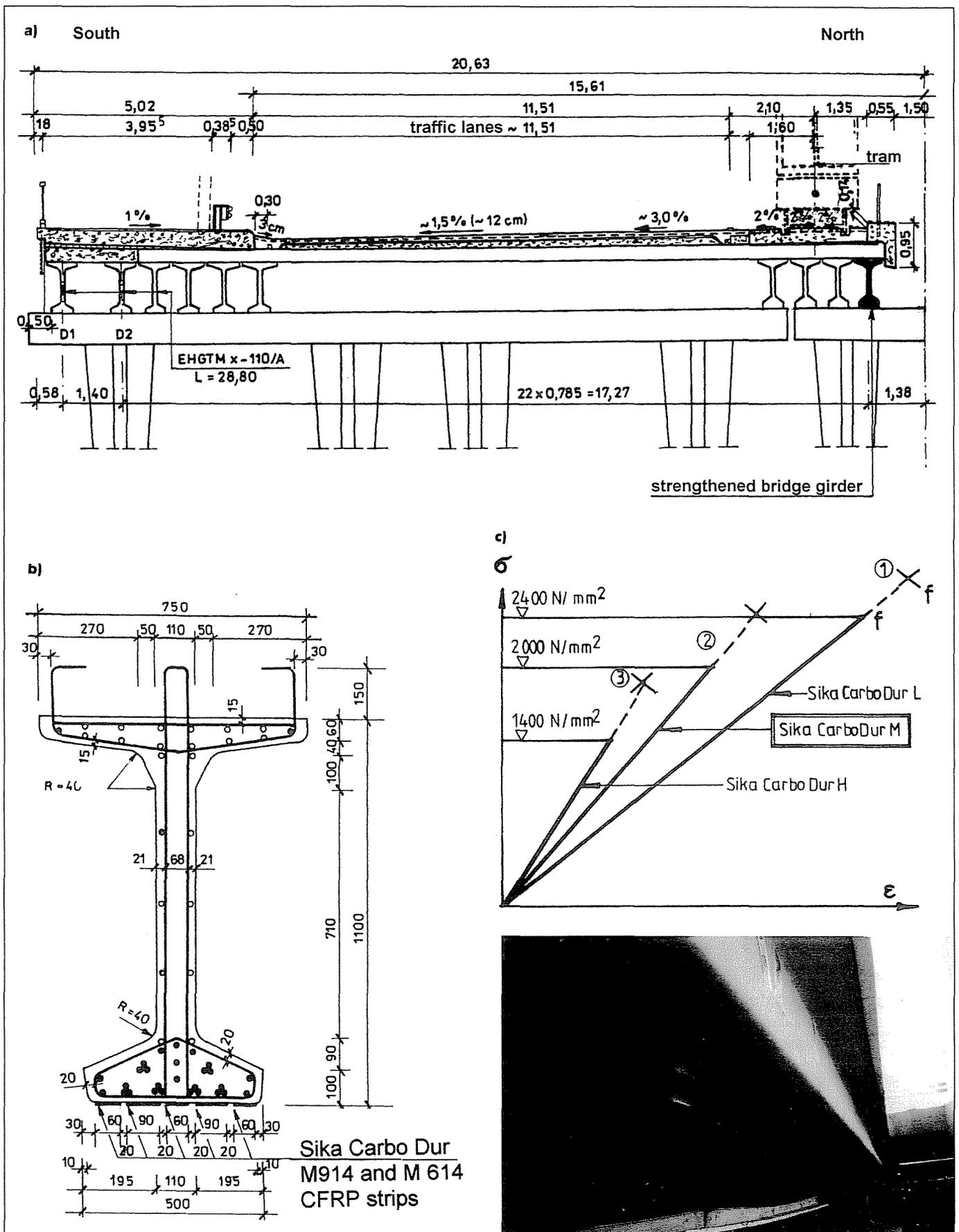
**Fig. 7** Strengthening of a prefabricated prestressed pre-tensioned concrete bridge girder in Budapest, Petöfi bridge owing to the failure of some prestressing strands due to corrosion. (Date: Sept. 1997, Strengthening strips: Sika CarboDur H914-56 m and M614-84 m. Designer: Budapest University of Technology; Dr. György L. Balázs and Dr. György Farkas. Exec: Pannon Freyssinet Ltd.)
