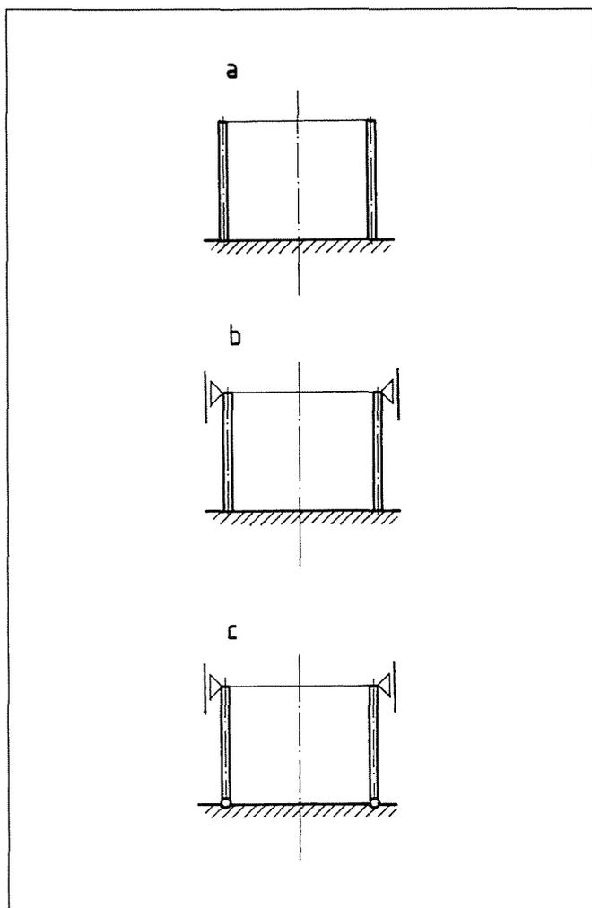
Fig. 3 Typical combinations of edge supports of the wall
