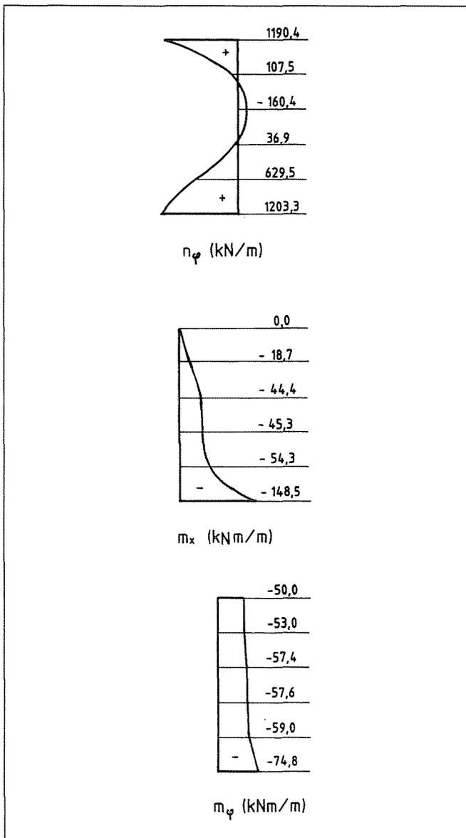
Fig. 4 Internal forces of a circular tank fixed at the bottom, hinged at the top ( $t_i = 0^\circ\text{C}$ ,  $t_o = -30^\circ\text{C}$ )
