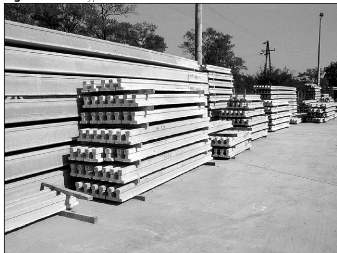
Fig. 2: Beams of type “EE” after manufacture
