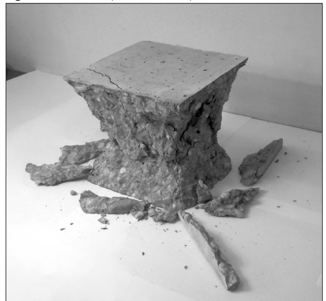
Fig. 1: Concrete cube specimen after compression test
