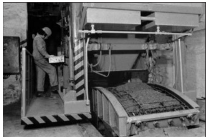
Fig. 22: Manufacturing equipment to prefabrication the tunnel lining segment elements
