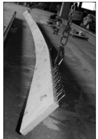
Fig. 12: The deformed shape of the experimental beam after the stability failure
