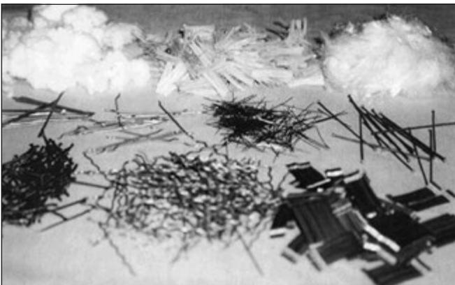
we studied how the 2 to 30 minute mixing of concrete influences the fibre properties of different fibre materials and fibre shapes.
