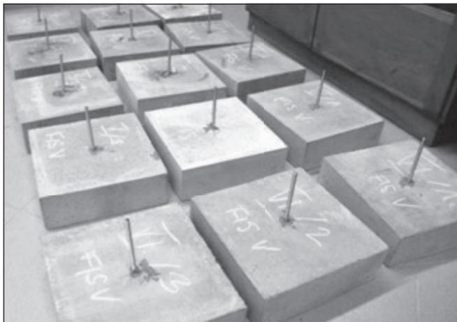
**Fig. 6:** Concrete specimens for pull-out tests
