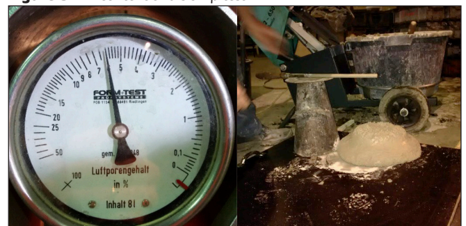
Figure 3. Air content and slump test
