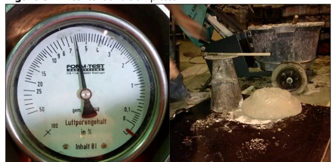
Figure 3. Air content and slump test
