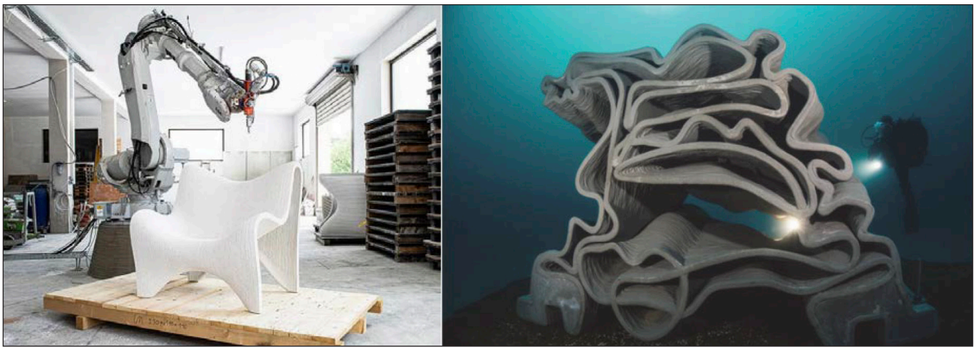
Fig. 14: Non-structural 3D printing concrete, (a) furniture (Aduatz, 2020), and (b) artificial underwater reefs (Xtree 2018)
