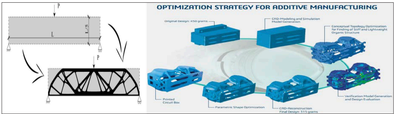
Fig. 6: Topological optimization concept, (a) simply supported beam subjected to load (Vantighem et. al., 2018), and (b) reduced amounts of materials during the design phase (Tripathy, 2016)
