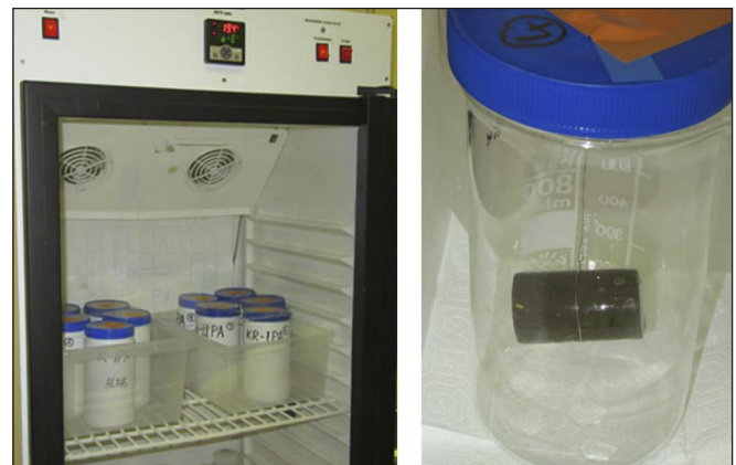
Fig. 4. The specimens stored in a climate chamber and the hanging leaching test specimen
