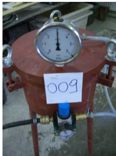
Fig. 2 Test apparatus (bleeding and filtration under pressure)
