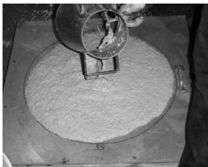
Fig. 3 Slump, “concrete cone”
