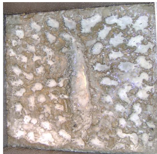
Fig. 4 Gypsum stamp to imprint equal surfaces Fig. 5 Imprinted accepting concrete surface
