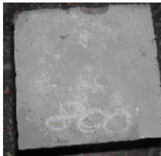
Fig. 7 Mono fibre reinforced concrete (800°C temperature load)
