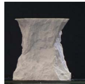
Fig. 2 Tested specimens with recycled glass
