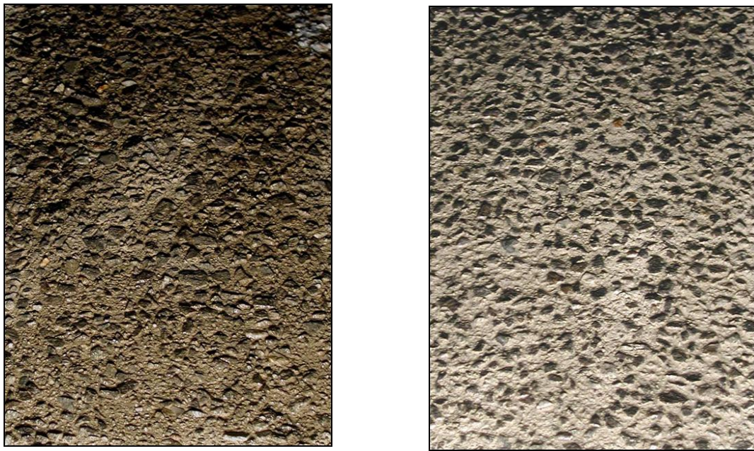
Fig. 4 Exposed aggregate concrete surfaces with dark aggregate (left) and exposed aggregate concrete surface with dark aggregate and titanium (II) oxide (right)
