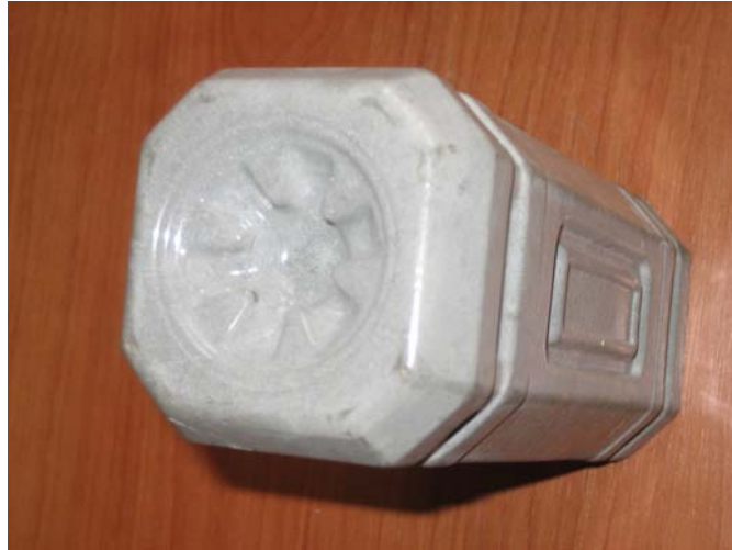
Fig. 5 SCC surface finishes
