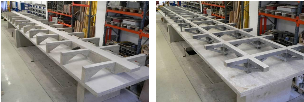
Fig. 6 Specimen 1 (left) and specimen 2 (right) after connection of the prefabricated elements
