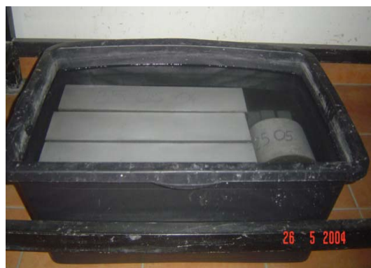
Fig. 1 Heat-treatment (left) and water curing (right)
