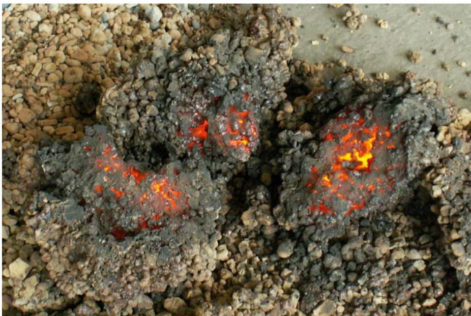
Fig. 1 The overburnt and insufficiently cooled batch
