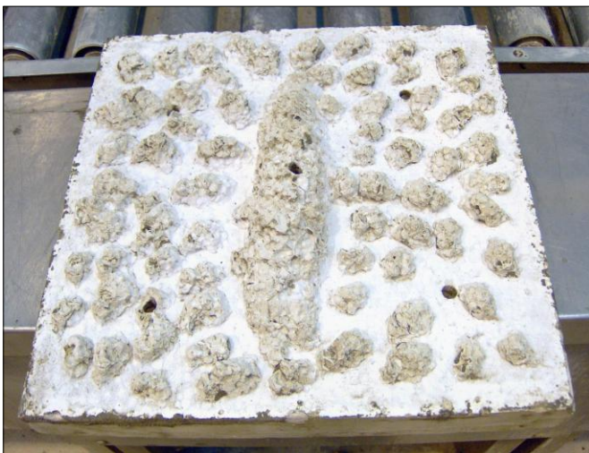
Fig. 4 Gypsum stamp to imprint equal surfaces Fig. 5 Imprinted accepting concrete surface
