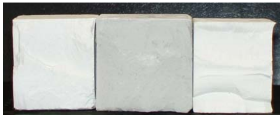
Fig. 5 Tested mortar mixtures: in the middle with limestone "00", at the sides with recycled glass
