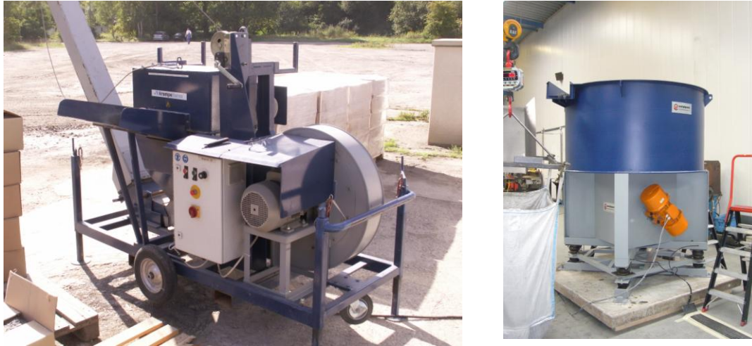
Fig. 1 Mixing and dosing machines for fibre reinforced concrete
