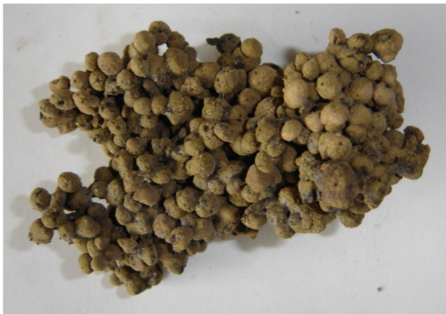
Fig. 2 The agglomerate of well burned grains
