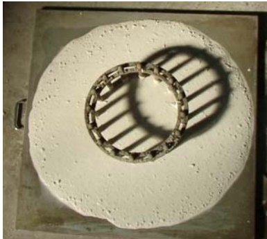
Fig. 7 Flow test of GBIII, with limestone and recycled glass, no carbon fiber added
