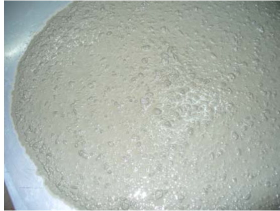
Fig. 4 SCC 17 – Slump-flow after VMA addition
