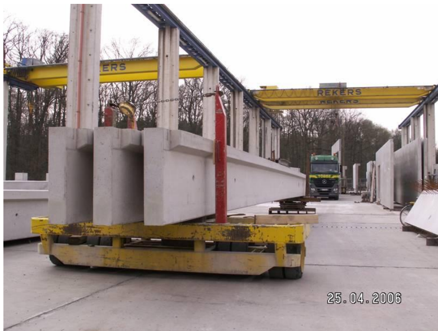
Fig. 3 Steel fibre reinforced beams for the IKEA Central Store
