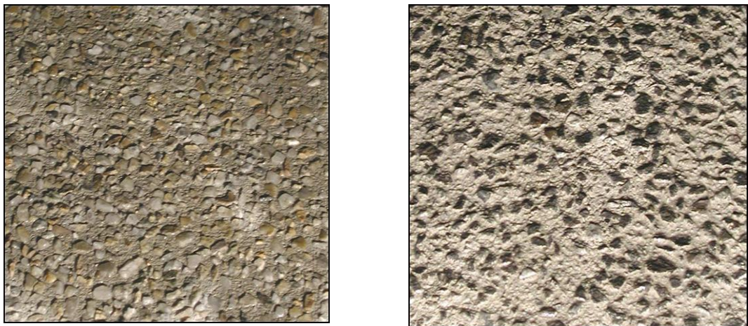
Fig. 5 Exposed aggregate concrete surface with bright aggregate (left) and exposed aggregate concrete surface with dark aggregate and titanium(II)oxide (right)
