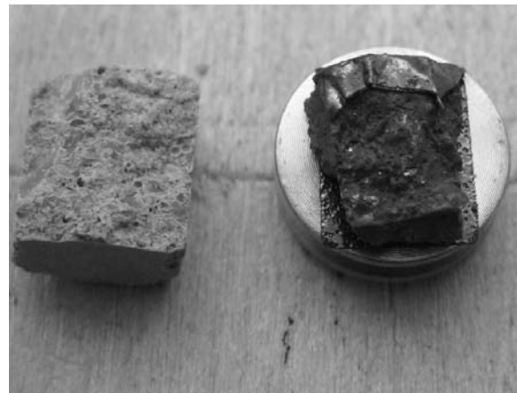
Fig. 2 SEM specimen - raw (left) and gold-coated (right)
