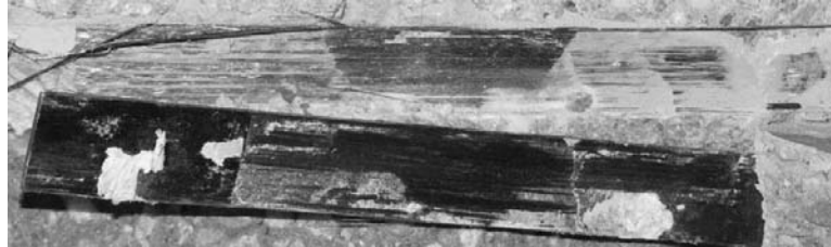
Fig. 3 Cohesive shear failure at FRP and adhesive interface
