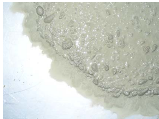
Fig. 3 SCC 17 – Slump-flow before VMA addition
