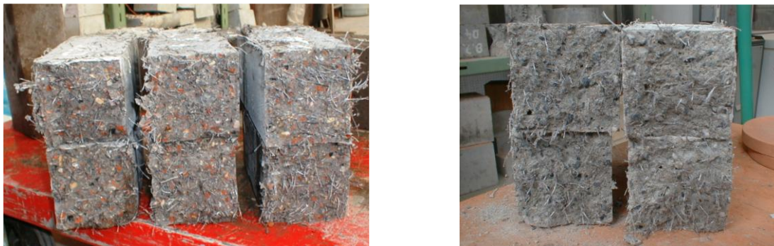
Fig. 2 Samples with fibers and recycled aggregates
