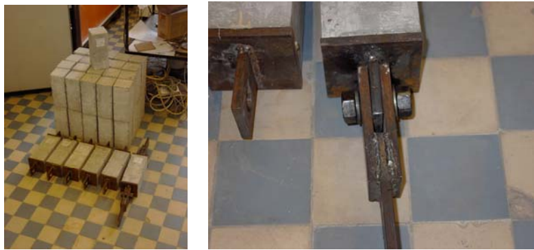
Fig. 4 Test specimens for uniaxial tensile test
