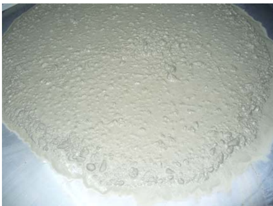
Fig. 3 SCC 17 – Slump-flow before VMA addition
