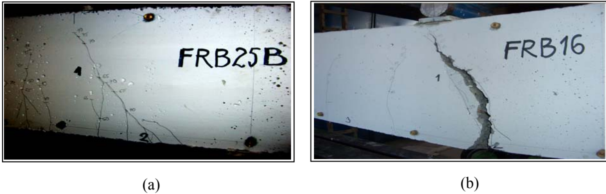
Fig. 4 (a) – Shear crack initiation, (b) – Beam failure
