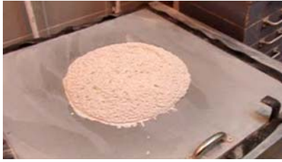
Fig. 3 Tested fresh concrete GB I., no recycled glass added
