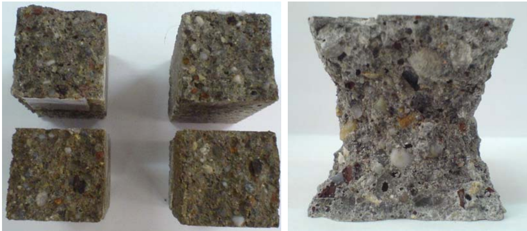
Fig. 2 Broken test pieces (left – bending; right – compressive tests)
