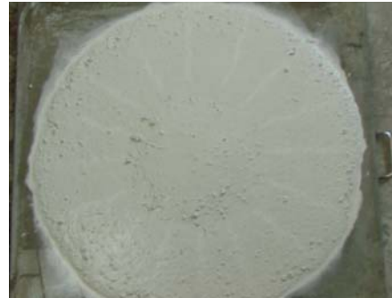
Fig. 8 Flow test of GBIV, with limestone and recycled glass, carbon fiber added
