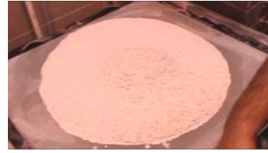
Fig. 4 Tested fresh concrete GB II., with recycled glass
