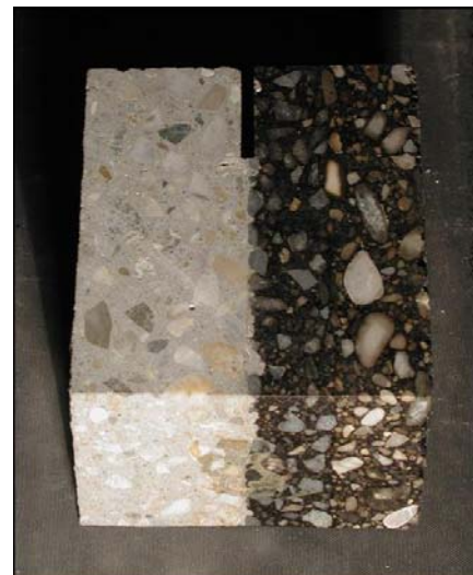
Fig. 2 Difference of the matrix by using homogenous aggregates
