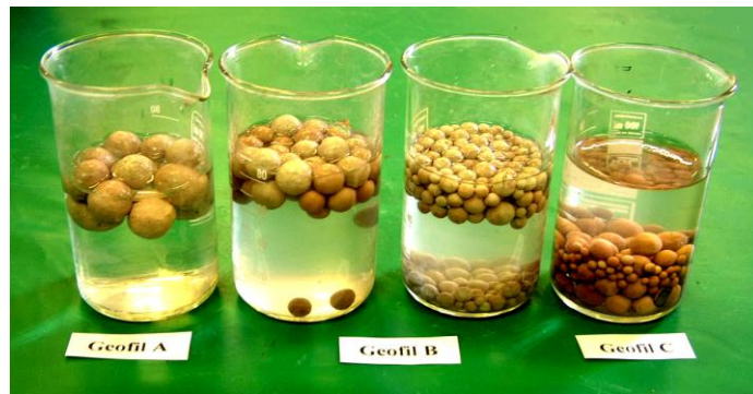
Fig. 6 Light weight aggregates with different diameters and densities (Józsa, Nemes, 2002)
