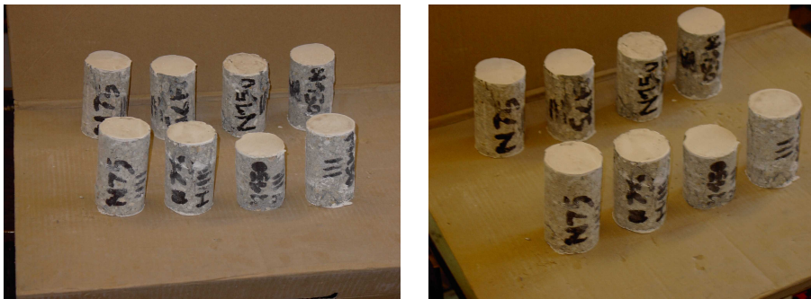
Photo 2.4: Failure of \varnothing=70 mm, \ell=100 mm cylinders in compression
