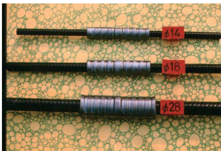
Fig. 1 Pressed sleeve splices
