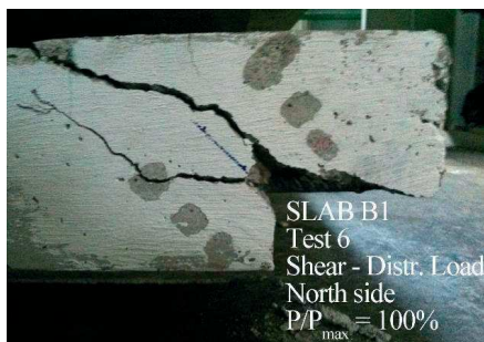
Fig. 8 Slab B1 with straight bars: Test No.6, distributed load, P_u = 172 kN
