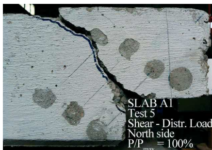
Fig. 7 Slab A1 with hooks and bent-up bars: Test No.5, distributed load, P_u = 401 kN
