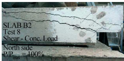
Fig. 10 Slab B2 with straight bars: Test No.8, concentrated load, P_u = 162 kN
