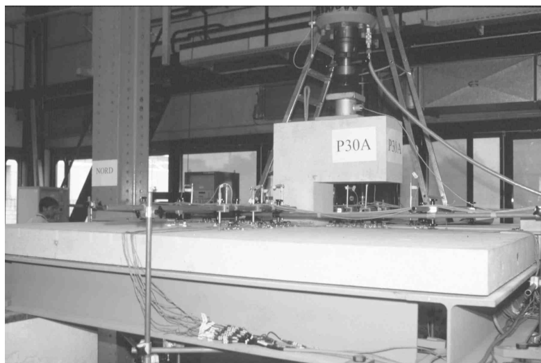
Fig. 3 Slab P30A during testing
